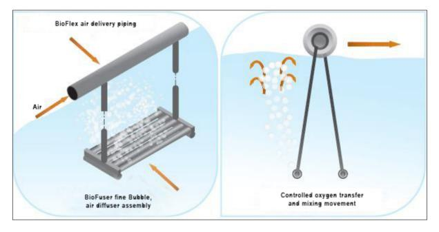
Figure 2: Fine Bubble Diffuser Mechanism
