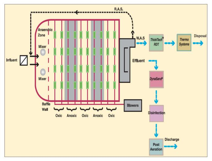
Figure 7: Wave Oxidation - Biological Nutrient Removal
